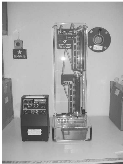
Coupled tanks with pump.
